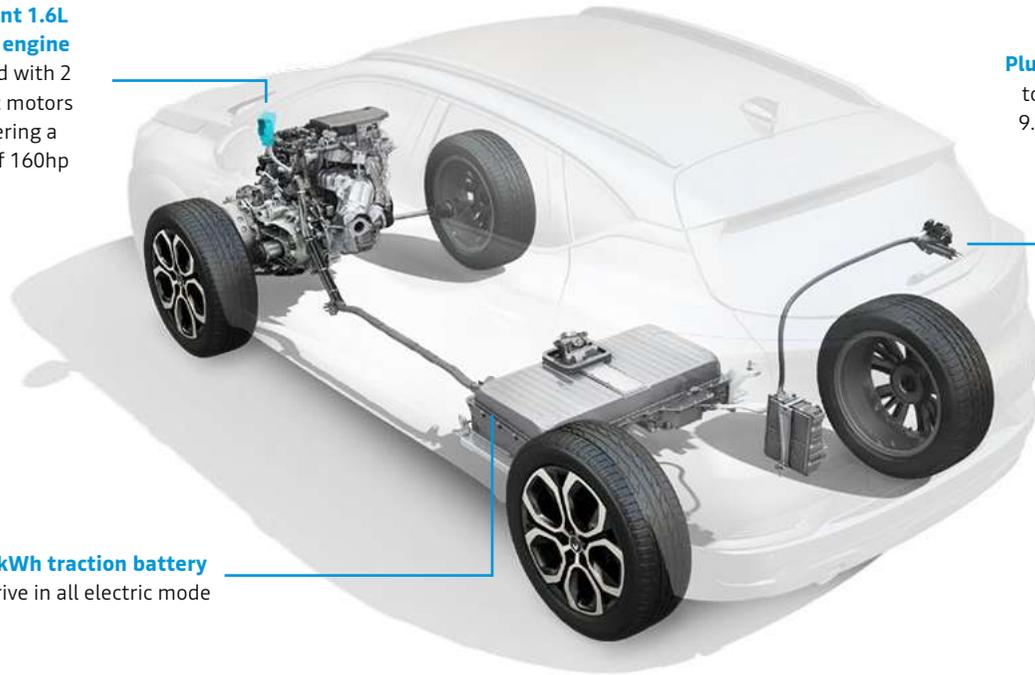
**Plug-in connector** to recharge the 9.8 kWh battery
